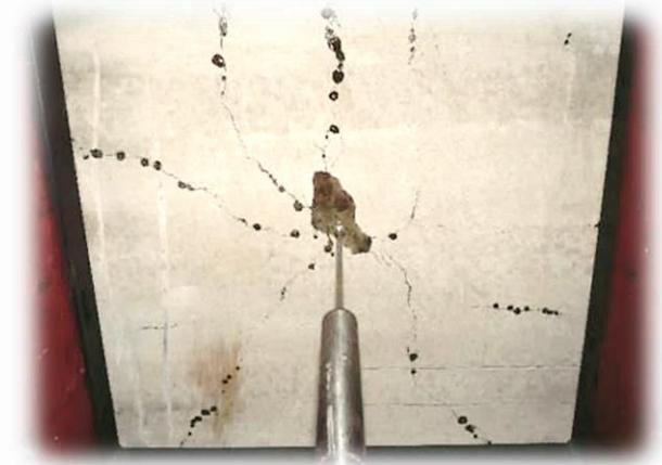
2D vascular network releasing sodium silicate in a 600 mm square concrete slab
